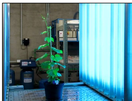
Irradiating a potted grapevine with UV-C light in the greenhouse at Hochschule Geisenheim University.
