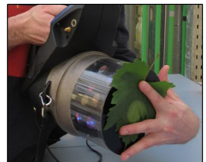
Using a Force-A Multiplex to measure the anthocyanin index in a grape leaf.
