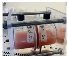
Double-compartment fermentation system consists of two glass chambers with loose screw caps, separated by a 0.45  $\mu m$  membrane filter obtained from VWR in Milan, Italy.
